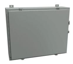
Hammond enclosure, NEMA 3R/4/12, 24 x 30 x 8in (HxWxD), wall mount, carbon steel, ANSI 61 gray, powder coat finish, single-door, stainless steel clamps, padlock hasp and staple.
