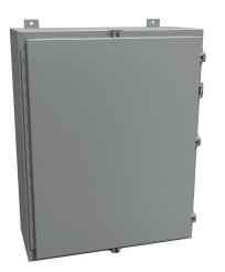
Hammond enclosure, NEMA 3R/4/12, 30 x 24 x 10in (HxWxD), wall mount, carbon steel, ANSI 61 gray, powder coat finish, single-door, stainless steel clamps, padlock hasp and staple.
