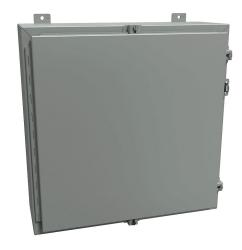
Hammond enclosure, NEMA 3R/4/12, 24 x 24 x 8in (HxWxD), wall mount, carbon steel, ANSI 61 gray, powder coat finish, single-door, stainless steel clamps, padlock hasp and staple.
