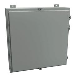
Hammond enclosure, NEMA 3R/4/12, 24 x 24 x 6in (HxWxD), wall mount, carbon steel, ANSI 61 gray, powder coat finish, single-door, stainless steel clamps, padlock hasp and staple.
