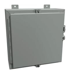
Hammond enclosure, NEMA 3R/4/12, 16 x 16 x 6in (HxWxD), wall mount, carbon steel, ANSI 61 gray, powder coat finish, single-door, stainless steel clamps, padlock hasp and staple.
