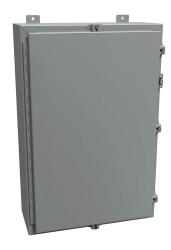
Hammond enclosure, NEMA 3R/4/12, 30 x 20 x 8in (HxWxD), wall mount, carbon steel, ANSI 61 gray, powder coat finish, single-door, stainless steel clamps, padlock hasp and staple.
