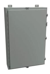
Hammond enclosure, NEMA 3R/4/12, 30 x 20 x 6in (HxWxD), wall mount, carbon steel, ANSI 61 gray, powder coat finish, single-door, stainless steel clamps, padlock hasp and staple.
