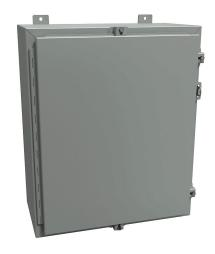
Hammond enclosure, NEMA 3R/4/12, 24 x 20 x 10in (HxWxD), wall mount, carbon steel, ANSI 61 gray, powder coat finish, single-door, stainless steel clamps, padlock hasp and staple.
