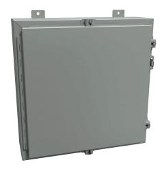
Hammond enclosure, NEMA 3R/4/12, 20 x 20 x 6in (HxWxD), wall mount, carbon steel, ANSI 61 gray, powder coat finish, single-door, stainless steel clamps, padlock hasp and staple.
