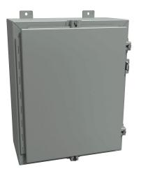
Hammond enclosure, NEMA 3R/4/12, 20 x 16 x 8in (HxWxD), wall mount, carbon steel, ANSI 61 gray, powder coat finish, single-door, stainless steel clamps, padlock hasp and staple.
