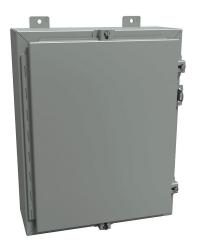
Hammond enclosure, NEMA 3R/4/12, 20 x 16 x 6in (HxWxD), wall mount, carbon steel, ANSI 61 gray, powder coat finish, single-door, stainless steel clamps, padlock hasp and staple.
