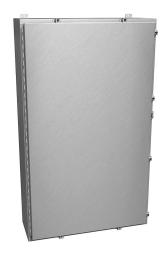
Hammond enclosure, NEMA 4/4X/12/13, 60 x 36 x 12in (HxWxD), wall mount, 5052-H32 aluminum, single-door, aluminum clamps, padlock hasp and staple.
