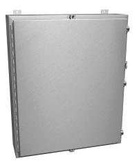
Hammond enclosure, NEMA 4/4X/12/13, 36 x 30 x 8in (HxWxD), wall mount, 5052-H32 aluminum, single-door, aluminum clamps, padlock hasp and staple.
