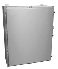
Hammond enclosure, NEMA 4/4X/12/13, 36 x 30 x 12in (HxWxD), wall mount, 5052-H32 aluminum, single-door, aluminum clamps, padlock hasp and staple.
