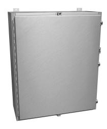
Hammond enclosure, NEMA 4/4X/12/13,  $36 \times 30 \times 12$ in (HxWxD), wall mount, 5052-H32 aluminum, single-door, aluminum clamps, padlock hasp and staple.
