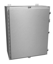
Hammond enclosure, NEMA 4/4X/12/13,  $30 \times 24 \times 12$ in (HxWxD), wall mount, 5052-H32 aluminum, single-door, aluminum clamps, padlock hasp and staple.
