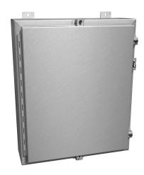
Hammond enclosure, NEMA 4/4X/12/13,  $24 \times 20 \times 6$ in (HxWxD), wall mount, 5052-H32 aluminum, single-door, aluminum clamps, padlock hasp and staple.
