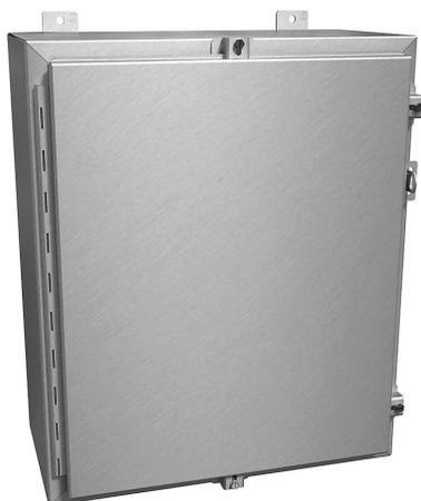
Hammond enclosure, NEMA 4/4X/12/13, 24 x 20 x 10in (HxWxD), wall mount, 5052-H32 aluminum, single-door, aluminum clamps, padlock hasp and staple.
