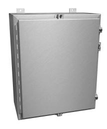
Hammond enclosure, NEMA 4/4X/12/13,  $24 \times 20 \times 10$ in (HxWxD), wall mount, 5052-H32 aluminum, single-door, aluminum clamps, padlock hasp and staple.
