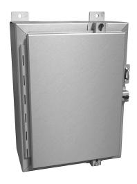
Hammond enclosure, NEMA 4/4X/12/13,  $16 \times 12 \times 6in$  (HxWxD), wall mount, 5052-H32 aluminum, single-door, aluminum clamps, padlock hasp and staple.
