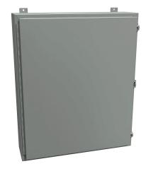
Hammond enclosure, NEMA 12/13, 36 x 30 x 8in (HxWxD), wall mount, carbon steel, ANSI 61 gray, powder coat finish, single-door, stainless steel clamps, padlock hasp and staple.
