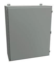
Hammond enclosure, NEMA 12/13, 36 x 30 x 12in (HxWxD), wall mount, carbon steel, ANSI 61 gray, powder coat finish, single-door, stainless steel clamps, padlock hasp and staple.
