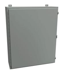
Hammond enclosure, NEMA 12/13, 36 x 30 x 10in (HxWxD), wall mount, carbon steel, ANSI 61 gray, powder coat finish, single-door, stainless steel clamps, padlock hasp and staple.
