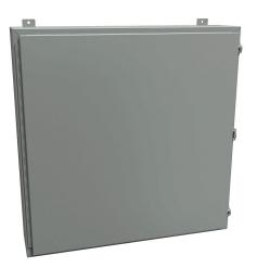
Hammond enclosure, NEMA 12/13, 36 x 36 x 8in (HxWxD), wall mount, carbon steel, ANSI 61 gray, powder coat finish, single-door, stainless steel clamps, padlock hasp and staple.
