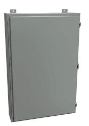
Hammond enclosure, NEMA 12/13, 36 x 24 x 6in (HxWxD), wall mount, carbon steel, ANSI 61 gray, powder coat finish, single-door, stainless steel clamps, padlock hasp and staple.
