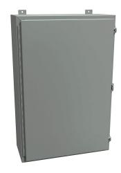
Hammond enclosure, NEMA 12/13, 36 x 24 x 10in (HxWxD), wall mount, carbon steel, ANSI 61 gray, powder coat finish, single-door, stainless steel clamps, padlock hasp and staple.
