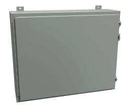
Hammond enclosure, NEMA 12/13, 24 x 30 x 8in (HxWxD), wall mount, carbon steel, ANSI 61 gray, powder coat finish, single-door, stainless steel clamps, padlock hasp and staple.
