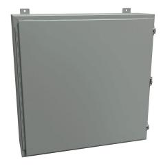
Hammond enclosure, NEMA 12/13, 30 x 30 x 8in (HxWxD), wall mount, carbon steel, ANSI 61 gray, powder coat finish, single-door, stainless steel clamps, padlock hasp and staple.
