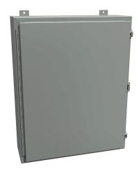
Hammond enclosure, NEMA 12/13, 30 x 24 x 8in (HxWxD), wall mount, carbon steel, ANSI 61 gray, powder coat finish, single-door, stainless steel clamps, padlock hasp and staple.
