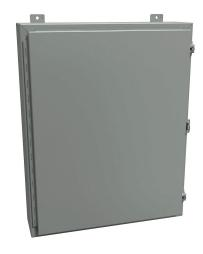
Hammond enclosure, NEMA 12/13, 30 x 24 x 6in (HxWxD), wall mount, carbon steel, ANSI 61 gray, powder coat finish, single-door, stainless steel clamps, padlock hasp and staple.
