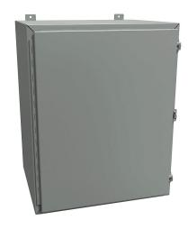
Hammond enclosure, NEMA 12/13, 30 x 24 x 20in (HxWxD), wall mount, carbon steel, ANSI 61 gray, powder coat finish, single-door, stainless steel clamps, padlock hasp and staple.
