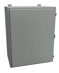
Hammond enclosure, NEMA 12/13, 30 x 24 x 16in (HxWxD), wall mount, carbon steel, ANSI 61 gray, powder coat finish, single-door, stainless steel clamps, padlock hasp and staple.
