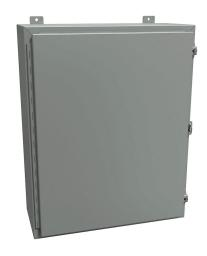
Hammond enclosure, NEMA 12/13, 30 x 24 x 10in (HxWxD), wall mount, carbon steel, ANSI 61 gray, powder coat finish, single-door, stainless steel clamps, padlock hasp and staple.
