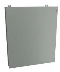
Hammond enclosure, NEMA 12,  $36 \times 30 \times 9$  in (HxWxD), wall mount, carbon steel, ANSI 61 gray, powder coat finish, hinged screw cover.
