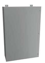
Hammond enclosure, NEMA 12, 36 x 24 x 9in (HxWxD), wall mount, carbon steel, ANSI 61 gray, powder coat finish, hinged screw cover.
