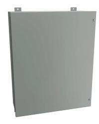
Hammond enclosure, NEMA 12, 30 x 24 x 9in (HxWxD), wall mount, carbon steel, ANSI 61 gray, powder coat finish, hinged screw cover.
