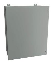
Hammond enclosure, NEMA 12,  $30 \times 24 \times 13$ in (HxWxD), wall mount, carbon steel, ANSI 61 gray, powder coat finish, hinged screw cover.
