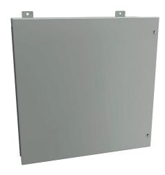
Hammond enclosure, NEMA 12, 24 x 24 x 9in (HxWxD), wall mount, carbon steel, ANSI 61 gray, powder coat finish, hinged screw cover.
