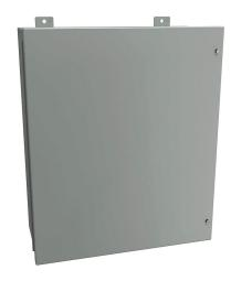
Hammond enclosure, NEMA 12, 24 x 20 x 9in (HxWxD), wall mount, carbon steel, ANSI 61 gray, powder coat finish, hinged screw cover.
