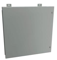
Hammond enclosure, NEMA 12, 20 x 20 x 7in (HxWxD), wall mount, carbon steel, ANSI 61 gray, powder coat finish, hinged screw cover.
