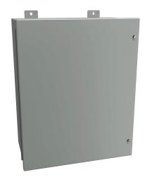
Hammond enclosure, NEMA 12, 20 x 16 x 9in (HxWxD), wall mount, carbon steel, ANSI 61 gray, powder coat finish, hinged screw cover.
