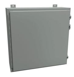
Hammond enclosure, NEMA 12/13, 24 x 24 x 8in (HxWxD), wall mount, carbon steel, ANSI 61 gray, powder coat finish, single-door, stainless steel clamps, padlock hasp and staple.
