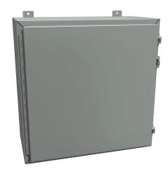
Hammond enclosure, NEMA 12/13, 24 x 24 x 12in (HxWxD), wall mount, carbon steel, ANSI 61 gray, powder coat finish, single-door, stainless steel clamps, padlock hasp and staple.
