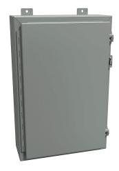
Hammond enclosure, NEMA 12/13, 24 x 16 x 6in (HxWxD), wall mount, carbon steel, ANSI 61 gray, powder coat finish, single-door, stainless steel clamps, padlock hasp and staple.
