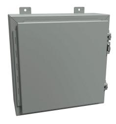
Hammond enclosure, NEMA 12/13, 16 x 16 x 6in (HxWxD), wall mount, carbon steel, ANSI 61 gray, powder coat finish, single-door, stainless steel clamps, padlock hasp and staple.
