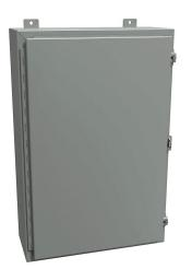
Hammond enclosure, NEMA 12/13, 30 x 20 x 8in (HxWxD), wall mount, carbon steel, ANSI 61 gray, powder coat finish, single-door, stainless steel clamps, padlock hasp and staple.
