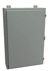
Hammond enclosure, NEMA 12/13, 30 x 20 x 6in (HxWxD), wall mount, carbon steel, ANSI 61 gray, powder coat finish, single-door, stainless steel clamps, padlock hasp and staple.
