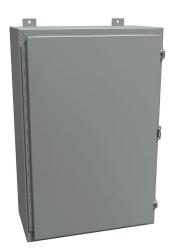
Hammond enclosure, NEMA 12/13, 30 x 20 x 10in (HxWxD), wall mount, carbon steel, ANSI 61 gray, powder coat finish, single-door, stainless steel clamps, padlock hasp and staple.
