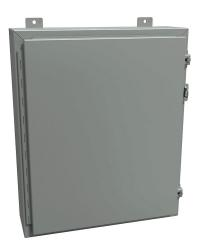
Hammond enclosure, NEMA 12/13, 24 x 20 x 6in (HxWxD), wall mount, carbon steel, ANSI 61 gray, powder coat finish, single-door, stainless steel clamps, padlock hasp and staple.
