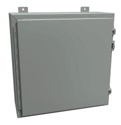
Hammond enclosure, NEMA 12/13, 20 x 20 x 8in (HxWxD), wall mount, carbon steel, ANSI 61 gray, powder coat finish, single-door, stainless steel clamps, padlock hasp and staple.
