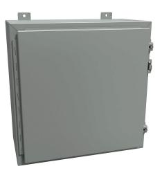
Hammond enclosure, NEMA 12/13, 20 x 20 x 10in (HxWxD), wall mount, carbon steel, ANSI 61 gray, powder coat finish, single-door, stainless steel clamps, padlock hasp and staple.
