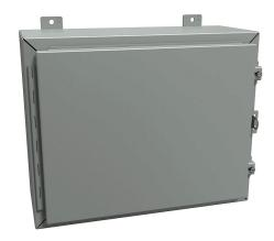
Hammond enclosure, NEMA 12/13, 16 x 20 x 8in (HxWxD), wall mount, carbon steel, ANSI 61 gray, powder coat finish, single-door, stainless steel clamps, padlock hasp and staple.
